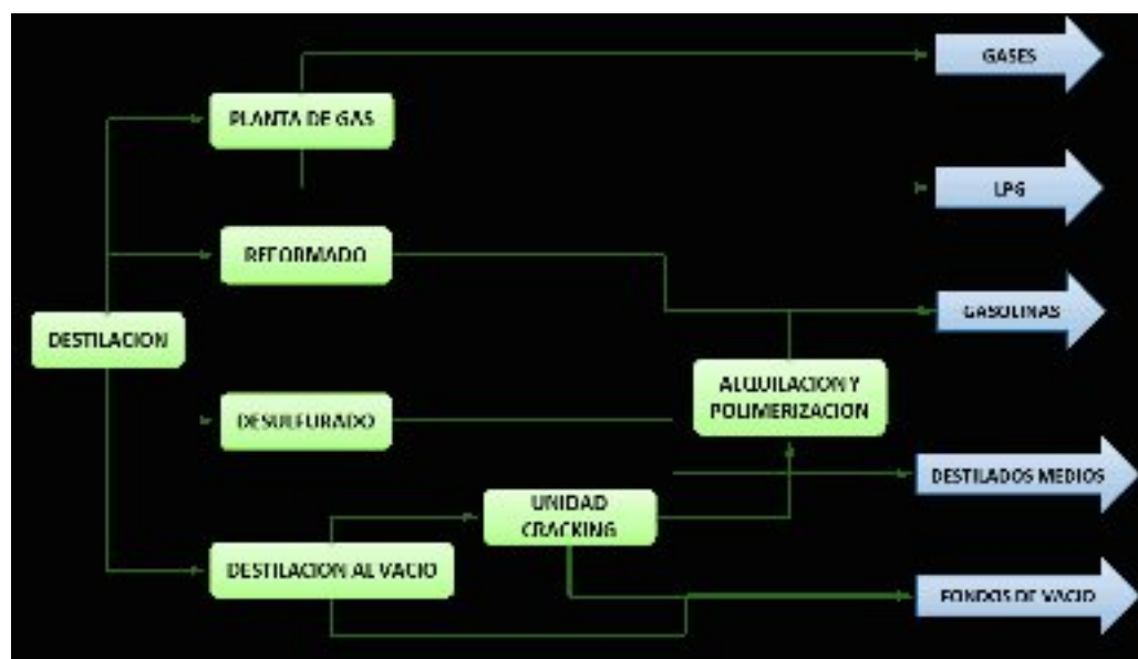
Illustration 2 – Distillation Scheme used by the Transporter
