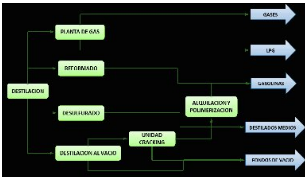
Illustration 2 – Distillation Scheme used by the Transporter
