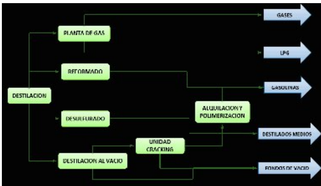
Illustration 2 – Distillation Scheme used by the Transporter
